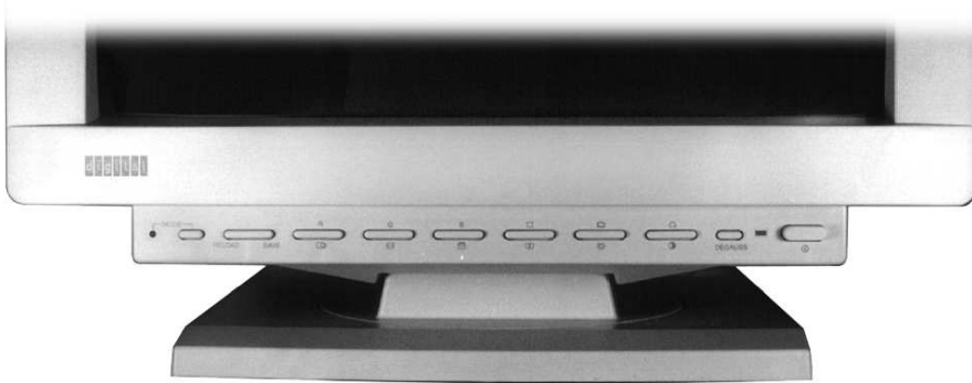
Figure 1-1 Monitor Control Panel
